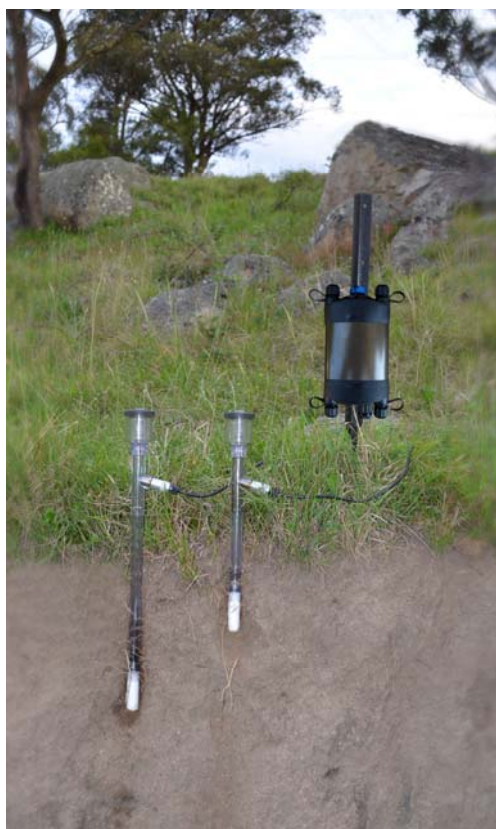
Jet Fill Tensiometers connected to the Soil Tension Meter
