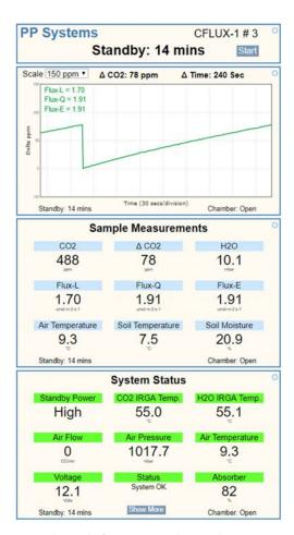
Sensor data and information is easily viewed via computor or mobile device. Flux rates based on linear, quadratic and exponential fit are continuously calculated and displayed.
