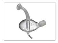
The Cyclonic Spray Chamber relies on momentum to efficiently and quickly remove the larger droplets from the sample mist decreasing any opportunity for occlusion or agglomeration of the smaller droplets. The result is higher efficiency, better precision and faster washouts than other spray chamber designs. For use with ball joint injectors.
