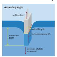
forces during the wetting and dewetting process versus the test liquids then supplies – either automatically or manually controlled – the dynamic advancing or receding contact angle, usually an important initial parameter to determine the surface energy.
