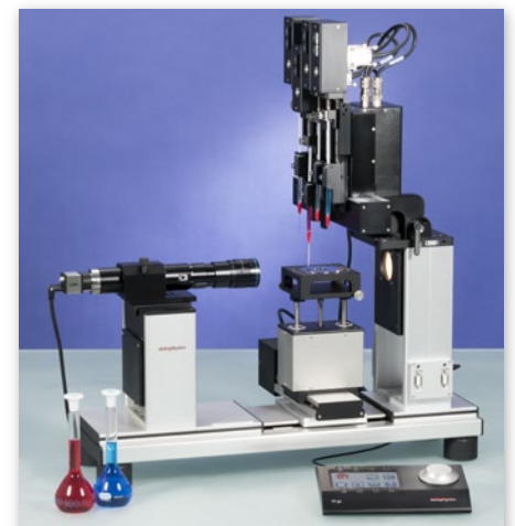
determination of the surface energy using an OCA 200 with DDE/4 and four ESr-N
