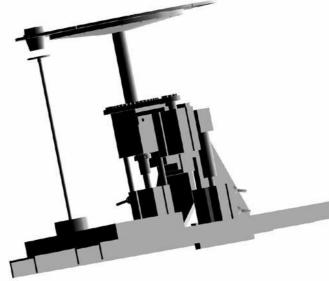
Single carousel configuration with manual placement & removal of crucible-covers for volatiles if used for coal (expandible to dual carousel, automatic crucible - covers)
