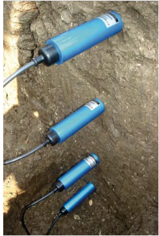
MP406 sensors installed in a soil profile
