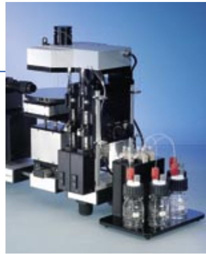
Refill and rinse system with liquid pump cleaner RRS-LPC 3/1 for OCA
