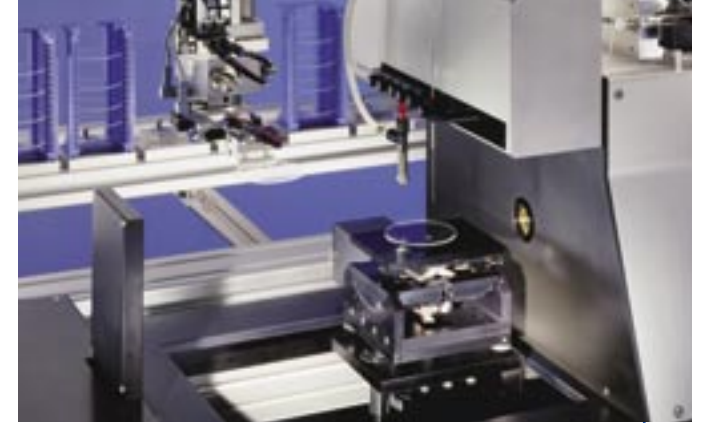
ACA 50 with the RCC robot system automatically loading coated glass wafers for measuring
