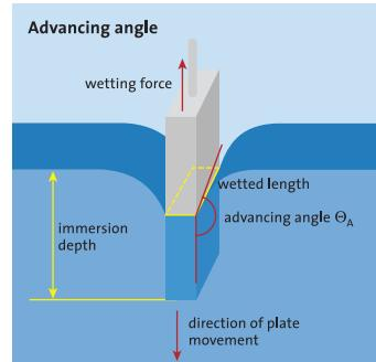
forces during the wetting and dewetting process versus the test liquids then supplies – either automatically or manually controlled – the dynamic advancing or receding contact angle, usually an important initial parameter to determine the surface energy.
