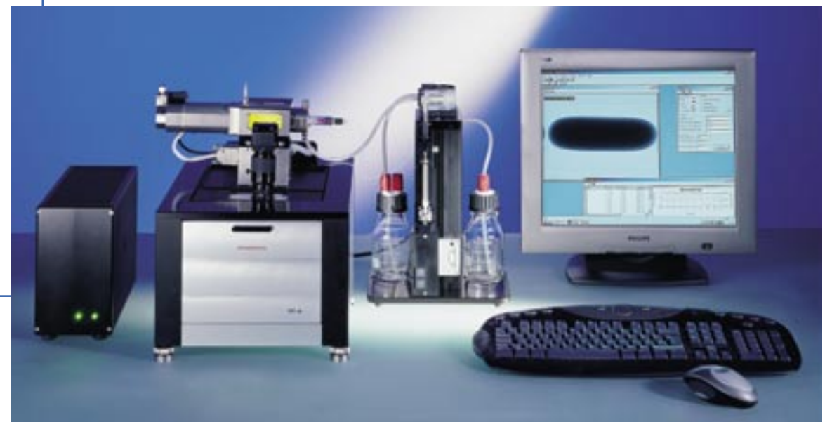
Spinning drop tensiometer SVT 20 with automatic dosing and refill system LDU / SVT
