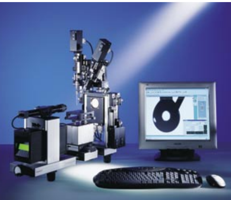
OCA 30 with the LIA-MD liquid injection system
