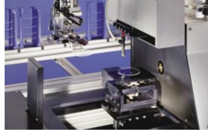
ACA 50 with the RCC robot system automatically loading coated glass wafers for measuring
