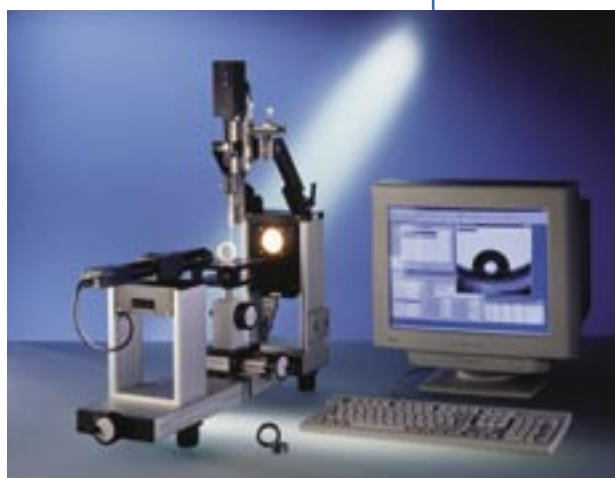
OCA 15 plus with SD-DM dosing system
