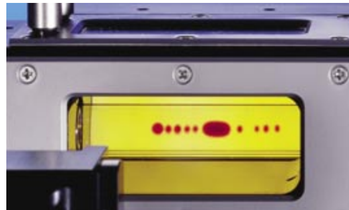
SVT 20 capillary with spinning drops
