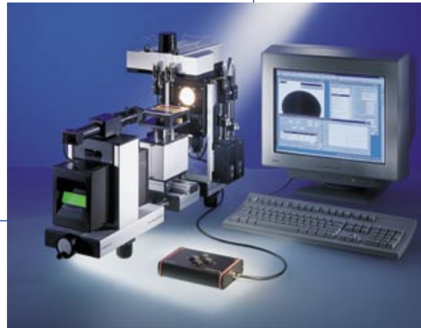
OCA 30 with E-MD/4 electronic dosing system and keypad
