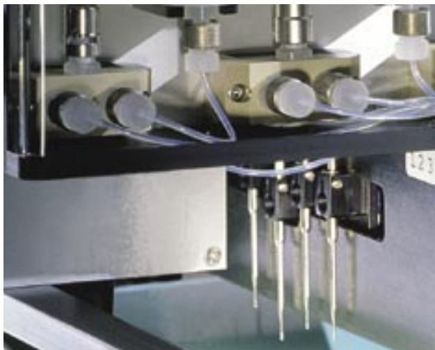
Dosing and refill system for the PCA 100M/4
