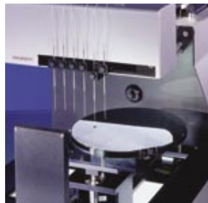
ACA 50 with wafer table and six electronic syringe units
