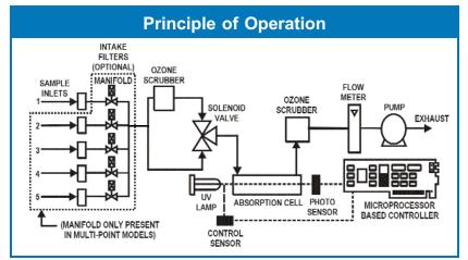
Measuring Principle: Absolute determination using UV
